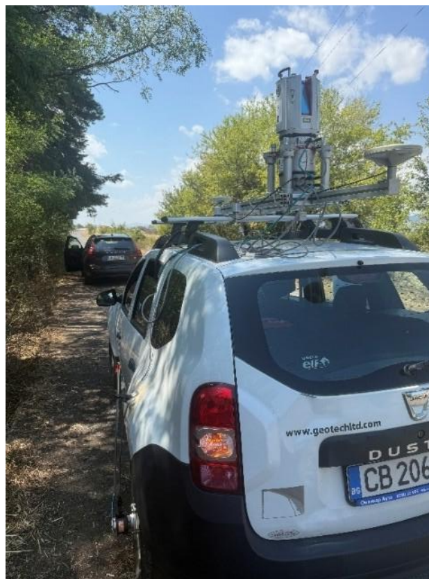
Figure 1. Integrated Laser System “RIEGL VMZ”
