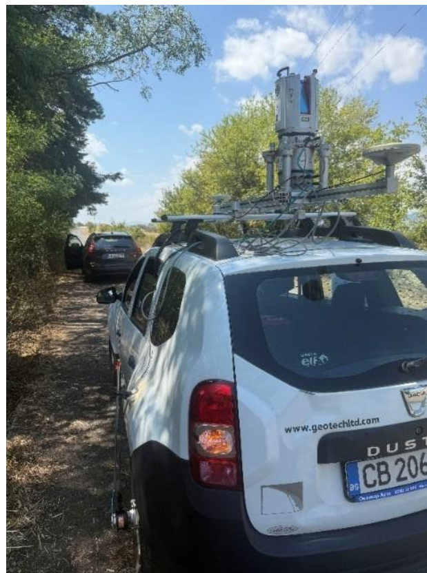
Figure 1. Integrated Laser System “RIEGL VMZ”
